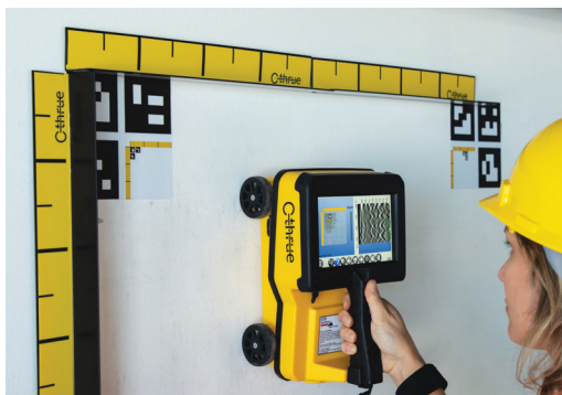
Automatic position and navigation system (Virtual Pad) increases productivity and reduces survey times.
